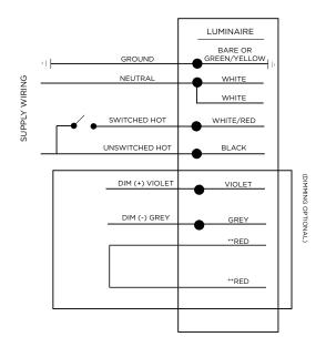
\*\* NOTE: DO NOT mate leads until installation is complete and AC power is supplied
