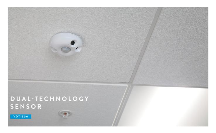
The Audacy® Dual-Technology Sensor is an AC line-powered, passive infrared and ultrasonic motion sensor. It can be used to detect occupancy and/or vacancy. The VDT1300 sends commands to control light fixtures equipped with Audacy Luminaire Controllers. Individual fixture control is available as well. The VDT1300 is mounted in the ceiling on a junction box.
