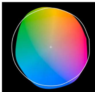
This Color Distortion Graphic of an LED light source shows the test light desaturates red hues, as well as some green and green-blue colors, while oversaturating green-yellows, blues and blue-purples.
