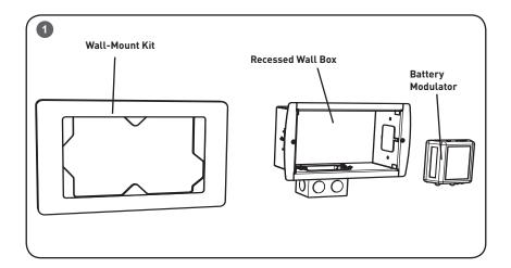
Installation of the provided recessed wall box, battery modulator, and wall-mount kit are required to complete the installation of the SmartCast® Touchscreen Control.
